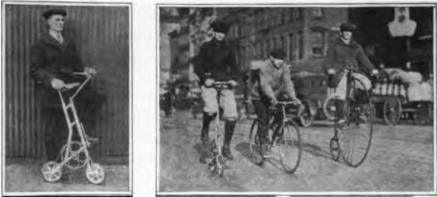
C. H. Clark's portable "city bicycle," in Scientific American , December 1919. The photograph on the right illustrates the inventor's confidence that his design would become the next evolutionary stage of the bicycle.
