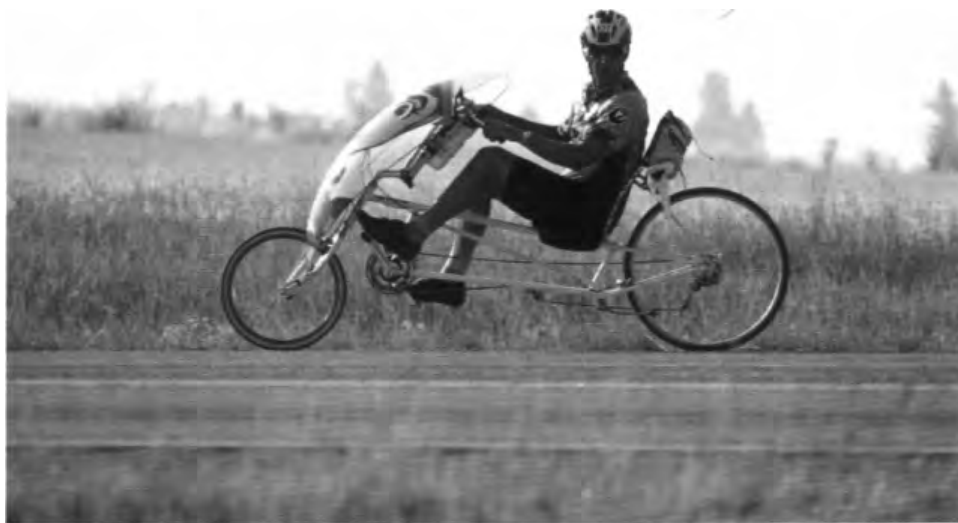
A semi-reclining recumbent with front fairing for streamlining. Proponents predict this style will become more popular with tourists looking to travel long distances in comfort.
