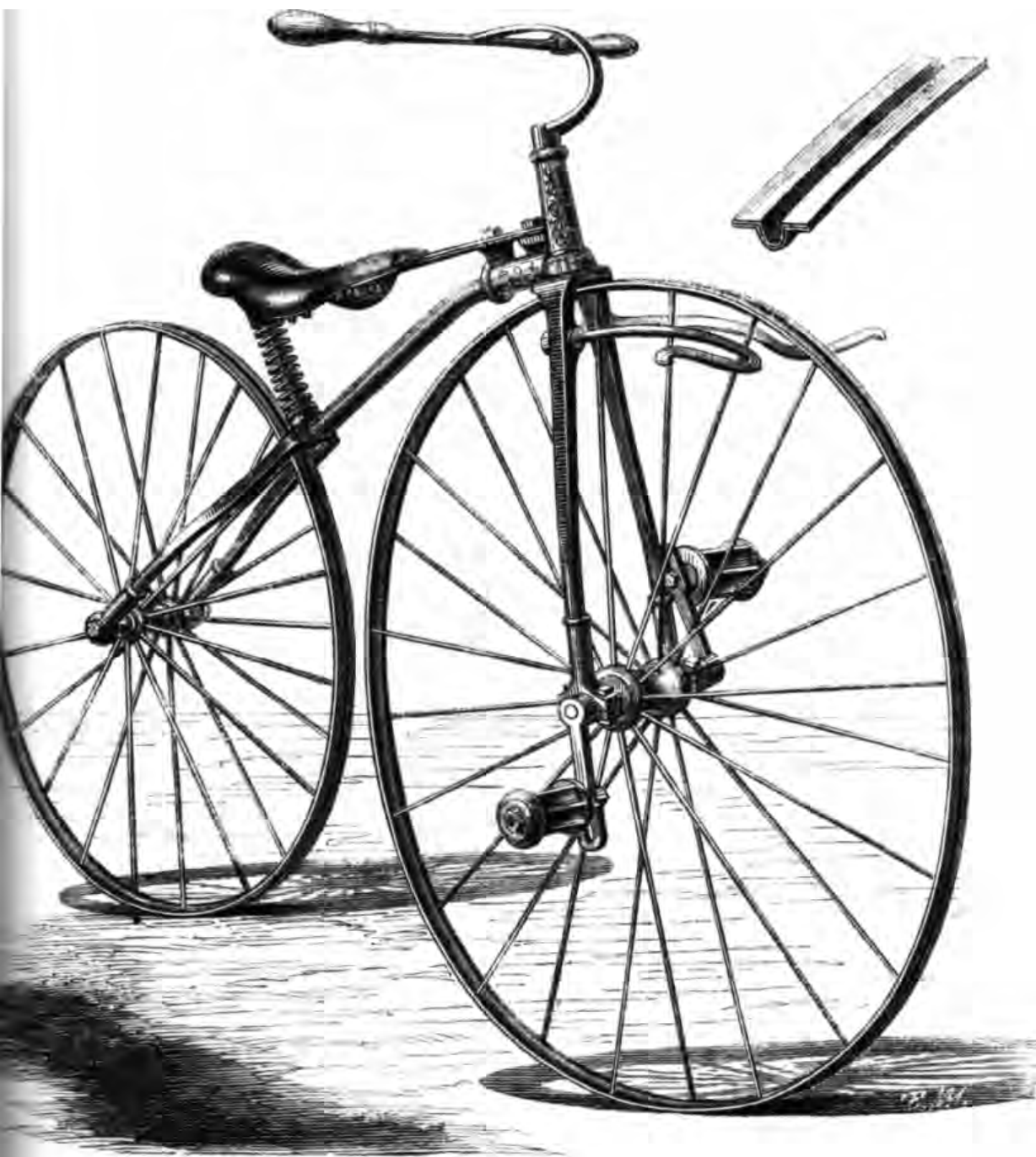
"Price's Improved Bicycle," featuring wire wheels patented by Virgil Price mounted on a Pickering frame, itself an advanced design, with finely engraved lugs. Wire wheels, a key improvement, were just beginning to appear in the United States when the velocipede craze fizzled. The inset in this sketch, which appeared in the Scientific American of 12 June 1869, shows how the iron rim is grooved to admit a rubber tire.
