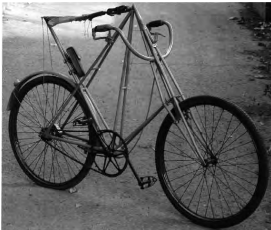
One of Mikael Pedersen's unusual bicycles weighing less than twenty pounds; this one from about 1898 featured a woven hammock seat for an especially comfortable ride. The rider could adjust a leather strap at the front of the seat to make it tighter or slacker according to taste. Even after the pneumatic tire greatly reduced road shock on conventional bicycles, there was still a modest demand for this model.
