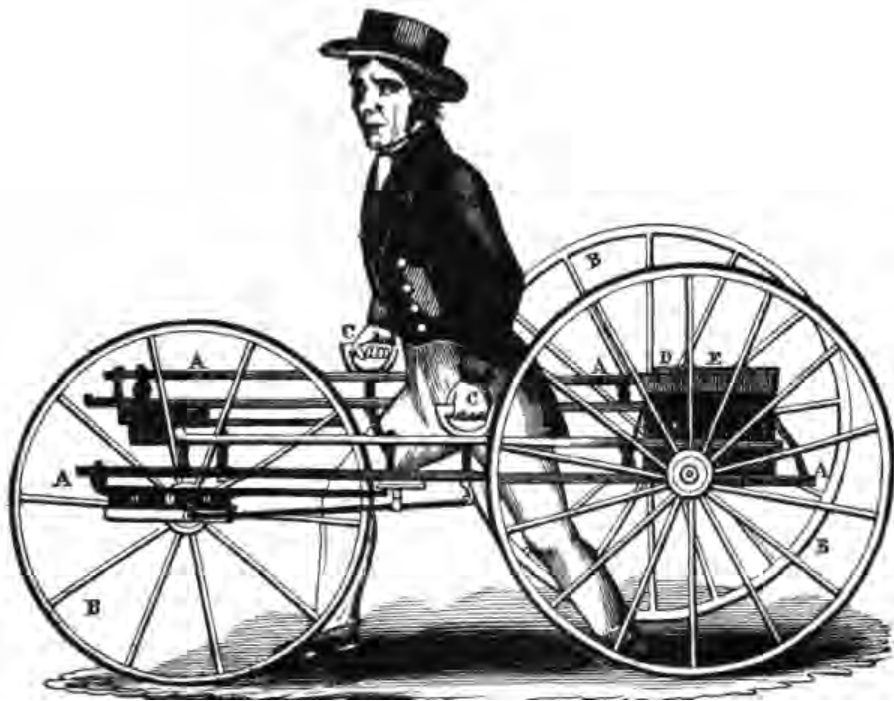
Gooch's Aeripedis, depicted in the Magazine of Science of 16 July 1842, was one of the few velocipedes of that period to retain Drais's kick-propulsion scheme. Like Drais, Gooch reluctantly concluded that mechanical drives were inherently inefficient.
